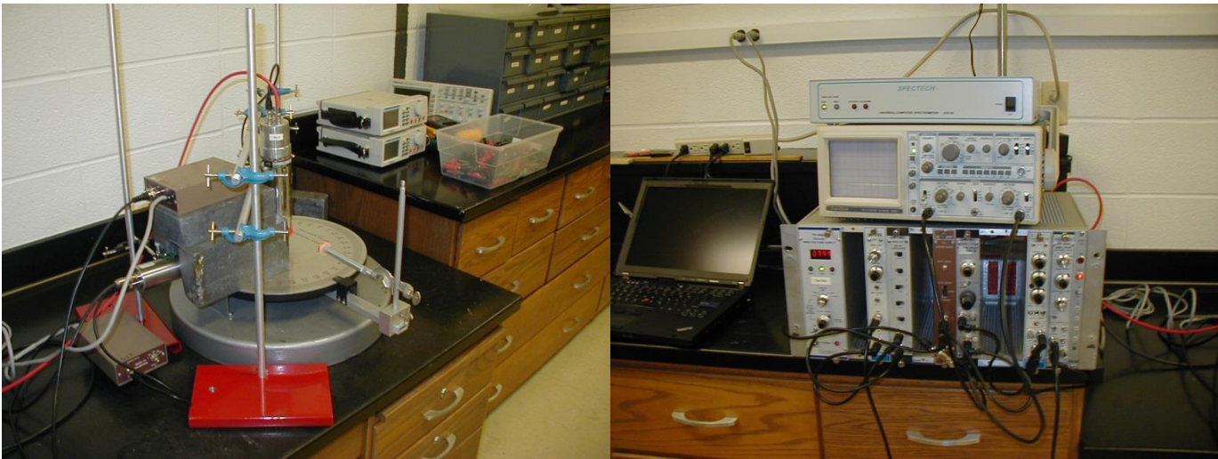
Figure 4 Photographs of the experimental apparatus showing (left) the gamma source attached to the movable arm, the NaI crystal active target, and the lead shielding which is surrounding the NaI detector for the scattered gamma rays, and (right) the NIM electronics and multichannel analyzer.
