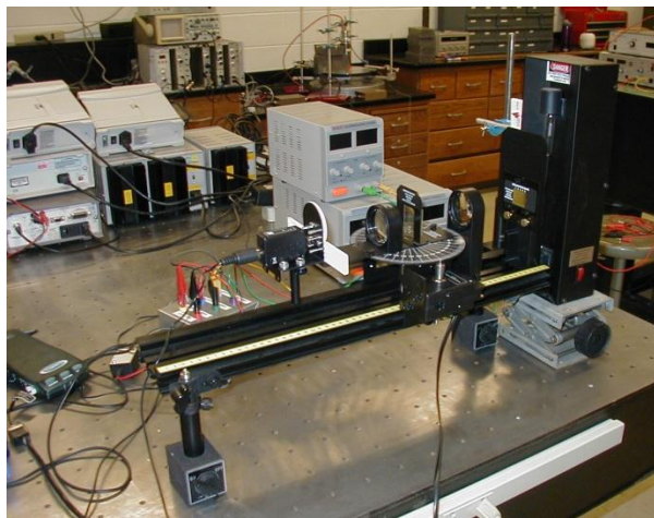
Figure 4. The spectrometer uses a diffraction grating to deflect light. The angle of deflection depends on the wavelength.
