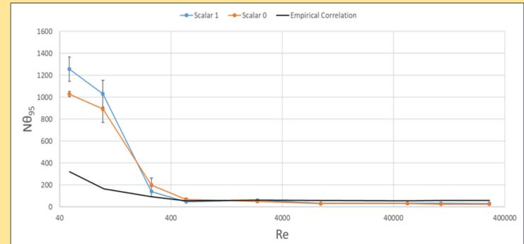
Figure 4: Non-dimensionalized mixing time as a function of the Reynolds number. Scalar 0 was initialized above the impeller away from the tank wall. Scalar 1 was initialized above the impeller in front of the baffle. Both scalar injection sites can be seen in Figure 3. Empirical correlations for laminar, transitional, and turbulent flow mixing (taken from Ref. [1]) are also plotted for comparison.
