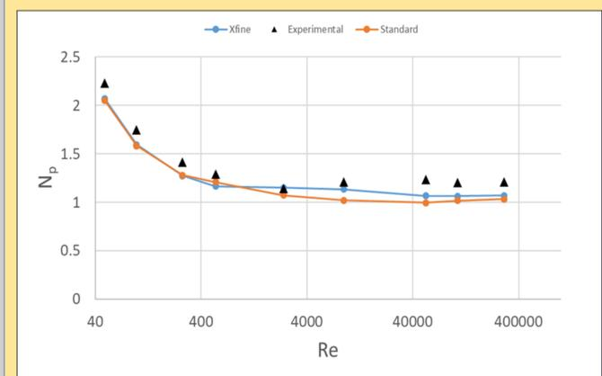
Figure 2: Power number results from simulations that used the standard mesh ("Standard") and the refined impeller mesh ("Xfine"). Results are compared to experimental data for the same system provided by SPX Flow.
