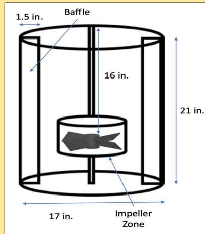
Figure 1: The tank and impeller geometries used in the present simulations. Note the center of the impeller is 16 inches from the top. The impeller diameter is 7 inches.
