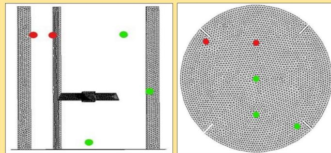
Figure 3: Two passive scalar injection sites (red) were used for predicting the mixing time. Concentration as a function of time was measured at three probe point locations (green). The left image provides a side view of the tank-impeller system and the right image is viewed from above.
