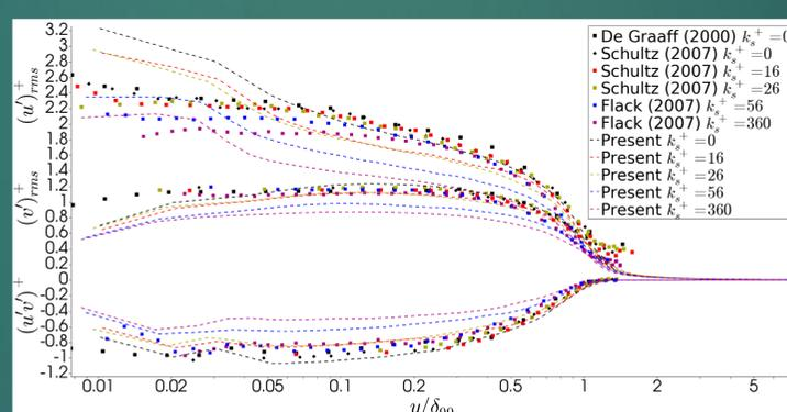
Figure 3. A plot of the Reynolds stresses nondimensionalized with respect to the friction velocity,  $u_{\tau}$ . In the figure,  $u'$  is the streamwise Reynolds stress,  $v'$  is the wall-normal Reynolds stress, and  $u'v'$  is the Reynolds shear stress.
