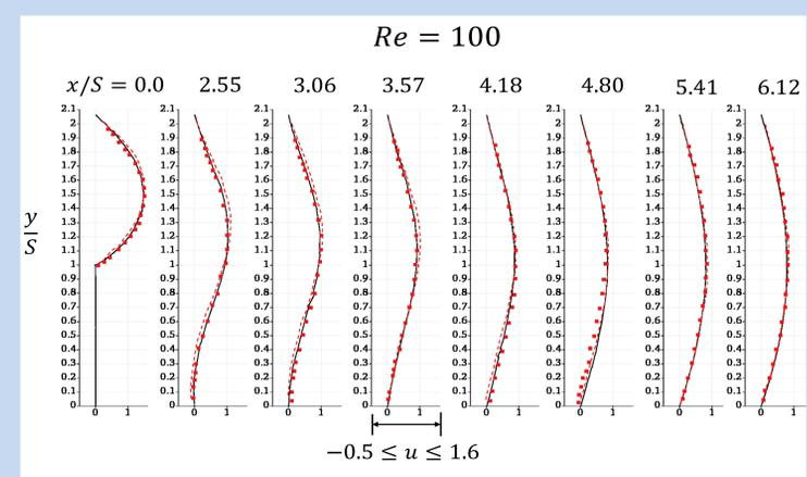
Figure 6. Axial velocity profiles at  $Re=100$  and different streamwise locations,  $x/S$ . The upstream channel ends at  $x/S=0$ . The solid black line, dotted red line and red squares are the present results, Chiang and Sheu data [5], and Armaly, et al. experimental data [4], respectively.
