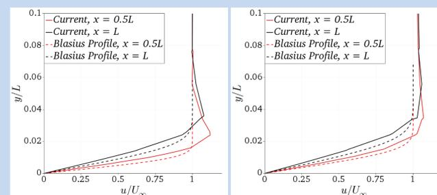
Figure 4. Velocity profiles for the full-sized (left) and shortened (right) grid cases. Profiles are shown at half the plate length and the full plate length. These are compared to the Blasius theory at the same position. The plots are shown with velocity on the  $x$ -axis and height above the wall on the  $y$ -axis.
