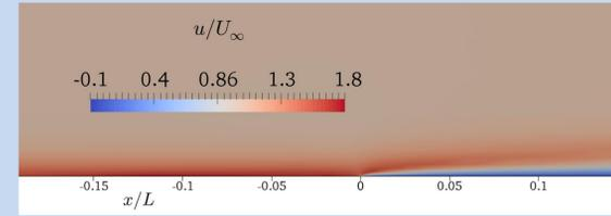
Figure 3. This figure shows contours of the axial velocity,  $u$ , normalized by the freestream velocity,  $U_\infty$ .  $x/L$  is the position in the axial direction, non-dimensionalized by the length of the plate – the plate begins at  $x/L = 0$ . This representative case uses  $P = 2$  and the coarsest grid tested.
