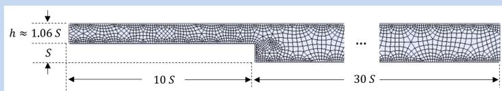
Figure 2. The geometry used for simulations of laminar channel flow over a backward-facing step.  $S$  is the height of the step and  $h$  is the upstream channel height. The flow is from left to right. The unstructured grid shown has approximately a third of the number of cells as the grid that is used here.
